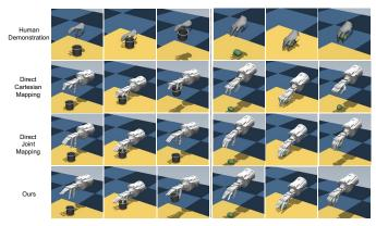
Fig. 6. Methods compared on the precision grasp task (left) and power grasp task (right).
