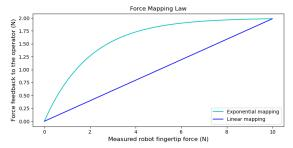
Fig. 4. Diagram of the force mapping law.
