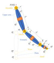
Fig. 3. Diagram of the human arm model.
