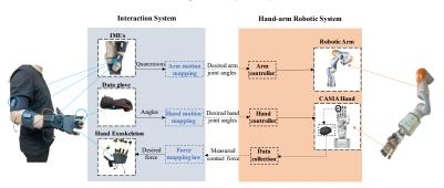
**Fig. 1.** The framework of human-like dexterous manipulation for the anthropomorphic hand-arm robotic system via teleoperation.
